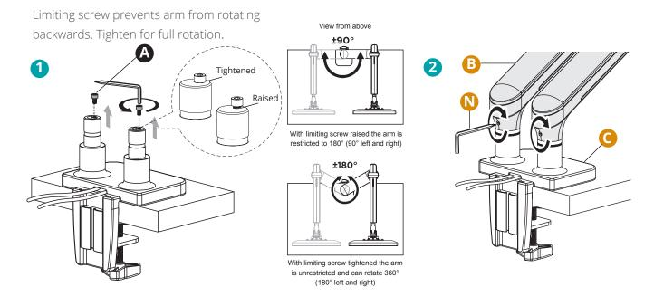
3 Take the upper arms A and slot the female connectors onto the male connections on the lower monitor arms B making sure they are fully inserted. Use the 4mm Allen key N and tighten the grub screw with the flat screwdriver end to lock the upper arms in place.
