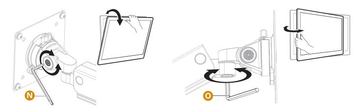
Swivel adjustment is factory set, however this can be adjusted using the **5mm Allen key ()** if required, turn the bolt clockwise to tighten or anti clockwise to loosen. Make small adjustments until the monitor is comfortable to move without feeling too loose.
