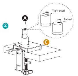
Limiting screw prevents arm from rotating backwards. Tighten for full rotation.
