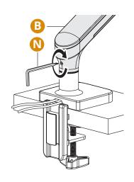
3 Take the upper arms (A) and slot the female connectors onto the male connections on the lower monitor arm (B) making sure they are fully inserted. Use the 4mm Allen key (N) and tighten the grub screw with the flat screwdriver end to lock the upper arms in place.
