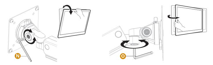
Swivel adjustment is factory set, however this can be adjusted using the **5mm Allen key ()** if required, turn the bolt clockwise to tighten or anti clockwise to loosen. Make small adjustments until the monitor is comfortable to move without feeling too loose.
