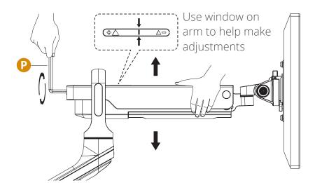
If arm rises turn adjustment screw to plus direction until monitor feels balanced to the weight of the monitor
